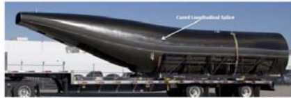
Figure 3: Example of load critical CFRP primary structure to be assembled by adhesive bonding: fuselage structures shall be joined by adhesive bonding
